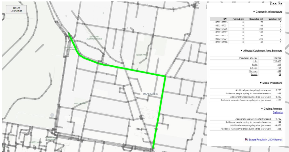
Figure 22. Hypothetical cycling path, Alison Road/Avoca Street – South scenario, (Approx. 1.1 km, estimated 1,321 new cyclists)
